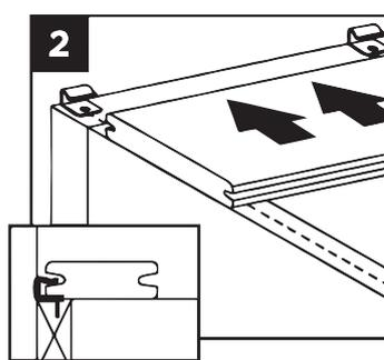
1. Install start clips on edge of ledger board, centred on each joist. Secure clips with screws.
