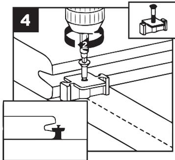
3. Insert fastener into grooved edge of deck board.
